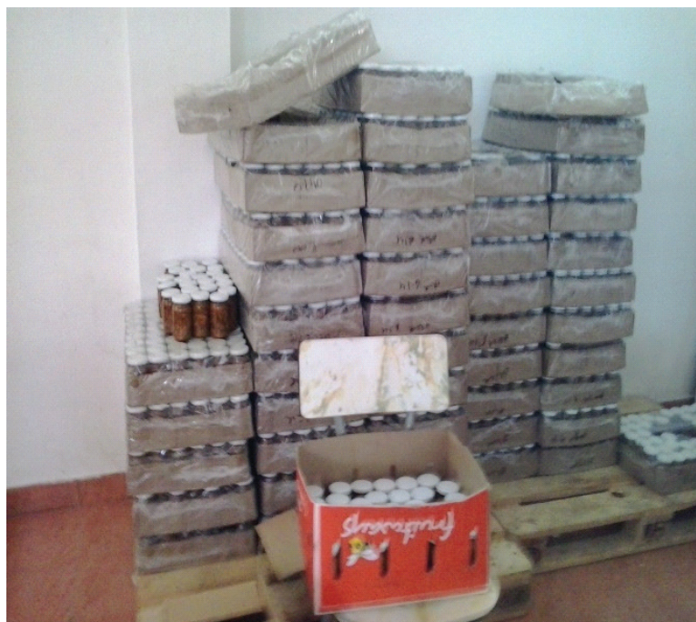
Figure 21: Jars stacked too high and in a haphazard way
